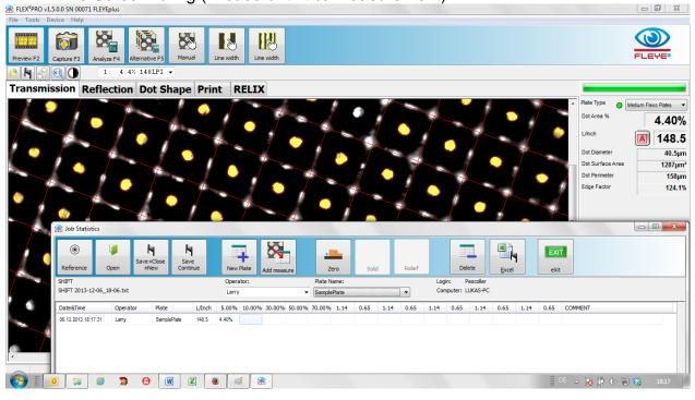
If the measurement is in tolerance, the value will be displayed on white background. In case it is out of tolerance the value will be displayed on red background.
